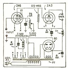
Fig. I. The basic circuit of the D.C. amplifier.
